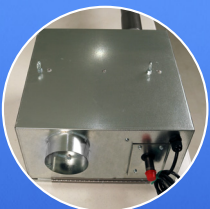
Air inlet relocated to follow heater tubes
