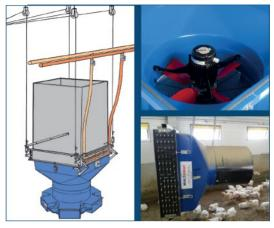
Hot water is supplied from an external boiler and passes the heat exchanger. The fan sucks the air from inside the building through the heat exchanger and pushes the warm air equally through the 6 air outlets in a horizontal flow over the birds. The amount of air and the directions can be adjusted by the optional flaps inside each air inlet. Hang the unit in the middle of the house to obtain ideal distribution to all corners in the building.
