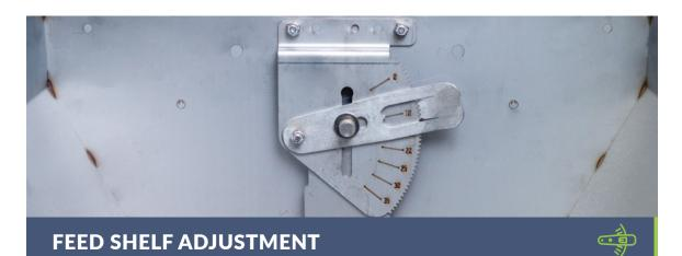
Adjust feed shelf settings as needed to provide 50-60% pan coverage (Figure 1). The feeder may need to be adjusted after each ration change to maintain the correct pan coverage.
